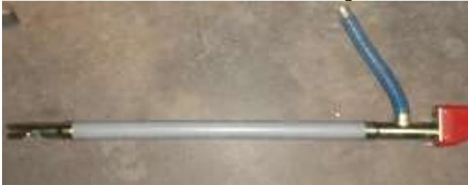
18. Assembled auger with hose mounted.
