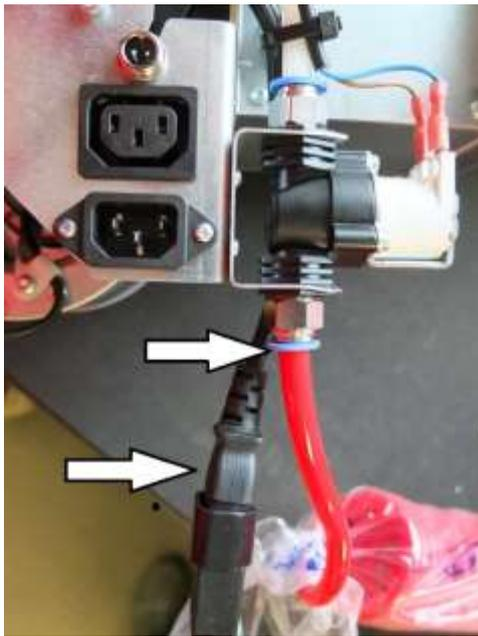
3. Assemble the compressor wire to the burner and attach the airhose onto the burner.
