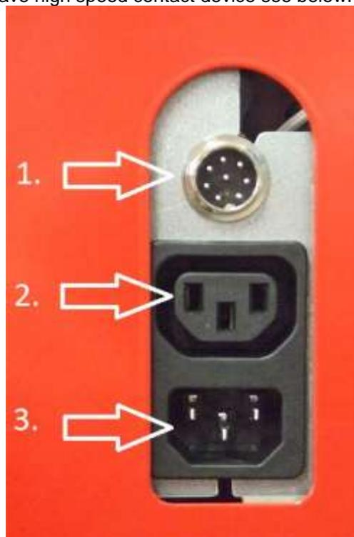
The protection cover of the burner can not be removed without pulling out all cables from the devices. The cable for supply voltage to the burner shall be connected by authorized electrician via the overheating protection of the boiler. Remaining connections have prepared cabling with connection devices that come with the burner.
