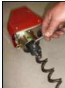
9. Fasten the outer the binding screw.
