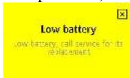
To close the alert screen, tap on . Closing the alert screen does not reset the alert. After closing the alert screen with , the alert code is still present in the upper left corner of the main screen as well as on all idle mode screens (see an example below).
