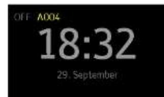
To see the alert message again, tap on the alert code in the upper left corner, in this example **A004**. To reset the alert, the issue must be solved. In this example, the battery must be replaced.
