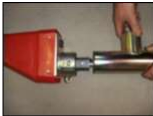
16. Push the auger pipe over the spiral and press on and fix it in place with the outlet of the T-pipe towards the side of the connector on the engine.
