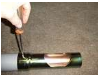
4. Fasten the plastic pipe and the metal inlet with the enclosed screw.
