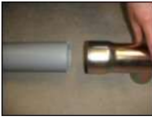
12. Push the plastic pipe together with the T-pipe in the opposite end you drilled the inlet hole in the plastic pipe.
