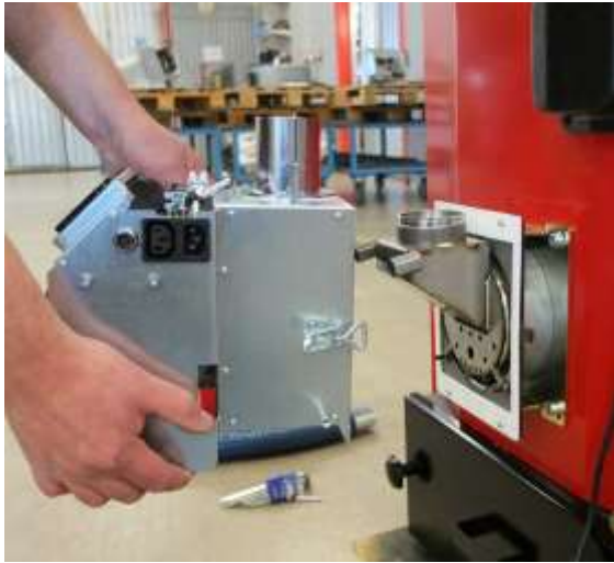
6. Lift the rear of the burner.
