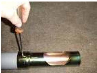
4. Fasten the plastic pipe and the metal inlet with the enclosed screw.
