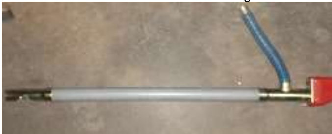
18. Assembled auger with hose mounted.
