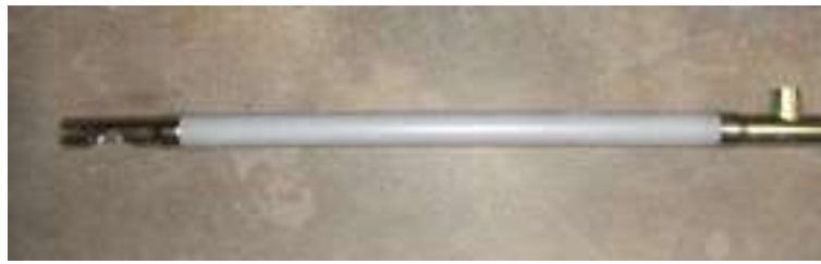
15. Auger pipe and T-pipe connected.
