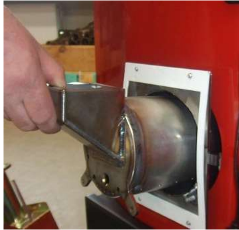
7. Pull out the inner chamber unit.
