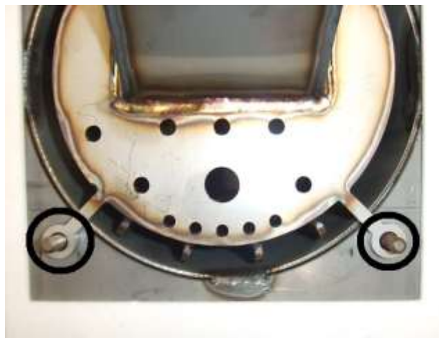
10. N.B ! When the inner chamber unit remounts it must be placed on both guide pins into the holes on the chamber unit.
