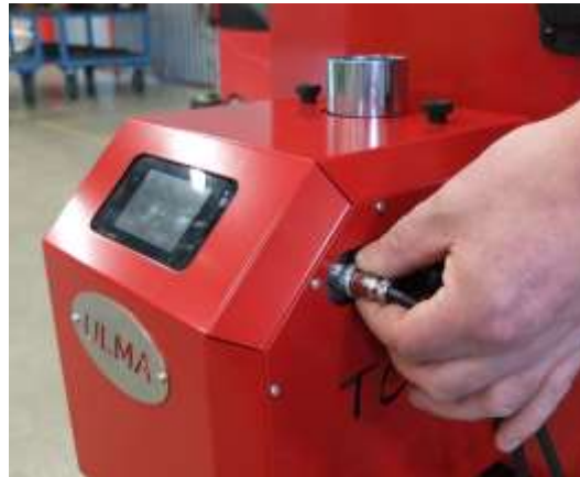
2. Press catch before pulling out temp sensor connector.
